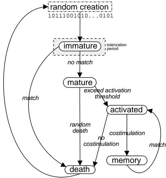
Figure 3: The lifecycle of a detector in LISYS.
